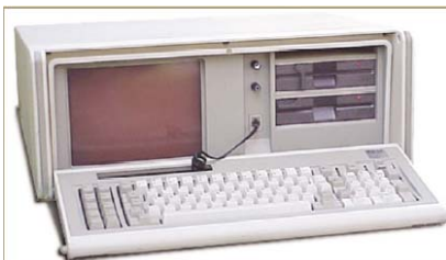
1984: IBM 5155 Intel 8088 at 4.77 MHz, $4225, amber monochrome monitor and no hard drive
