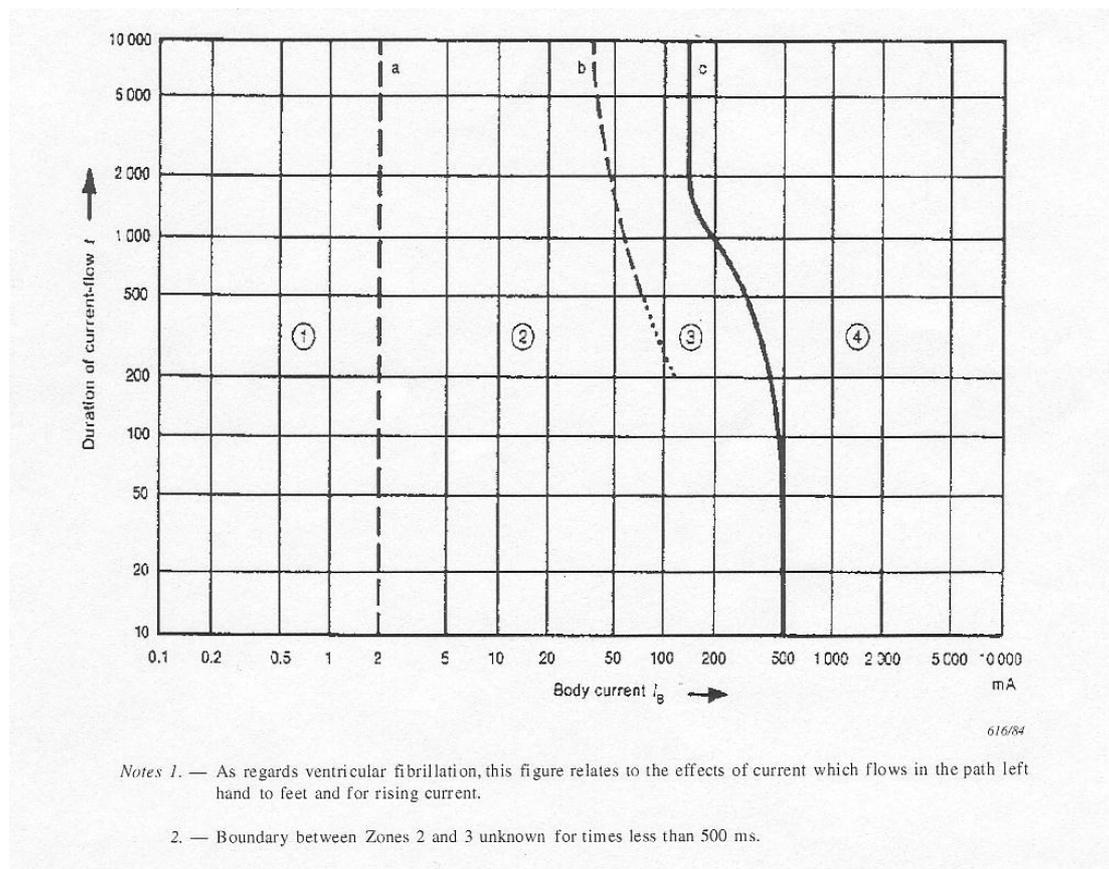
**Figure 5.4: Time/current zones for direct currents
