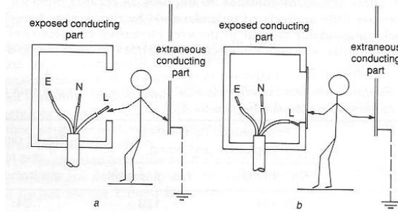
**Figure 5.1: Electric shock from exposed conductors**
