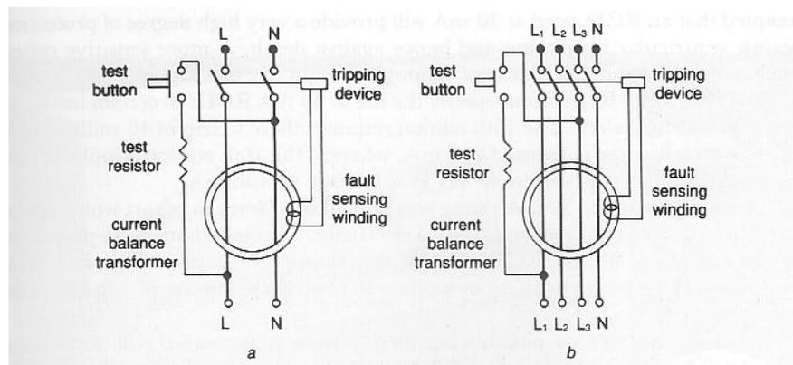
Figure 5.5: Diagrams showing the principle of the RCD to detect fault and leakage currents to earth and interrupt the supply
