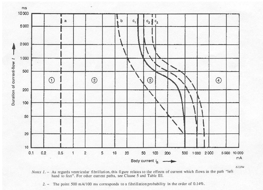
**Figure 5.3: Time/current zones of alternating currents (15 – 100 Hz) on persons (Standards Australia 1991, AS 3859:1991, p.15)**
